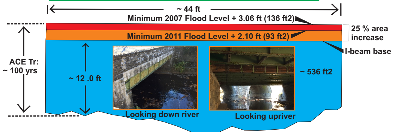
Channel cross-section beneath the Verdent Ave bridge
